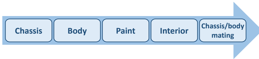
Fig. 5. Major Processes of a Car Assembly Line
